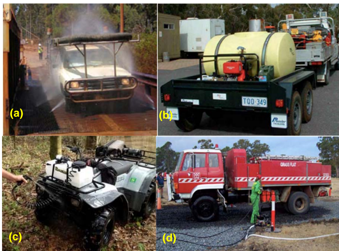
Figure 4. (a) A permanent automatic wash-down facility in Western Australia, (b) portable trailer wash-down unit, (c) All Terrain Vehicle (ATV) mounted with spray unit for washdown and (d) semi-permanent wash-down facility in Victoria (O’Gara et. al. 2005c)
