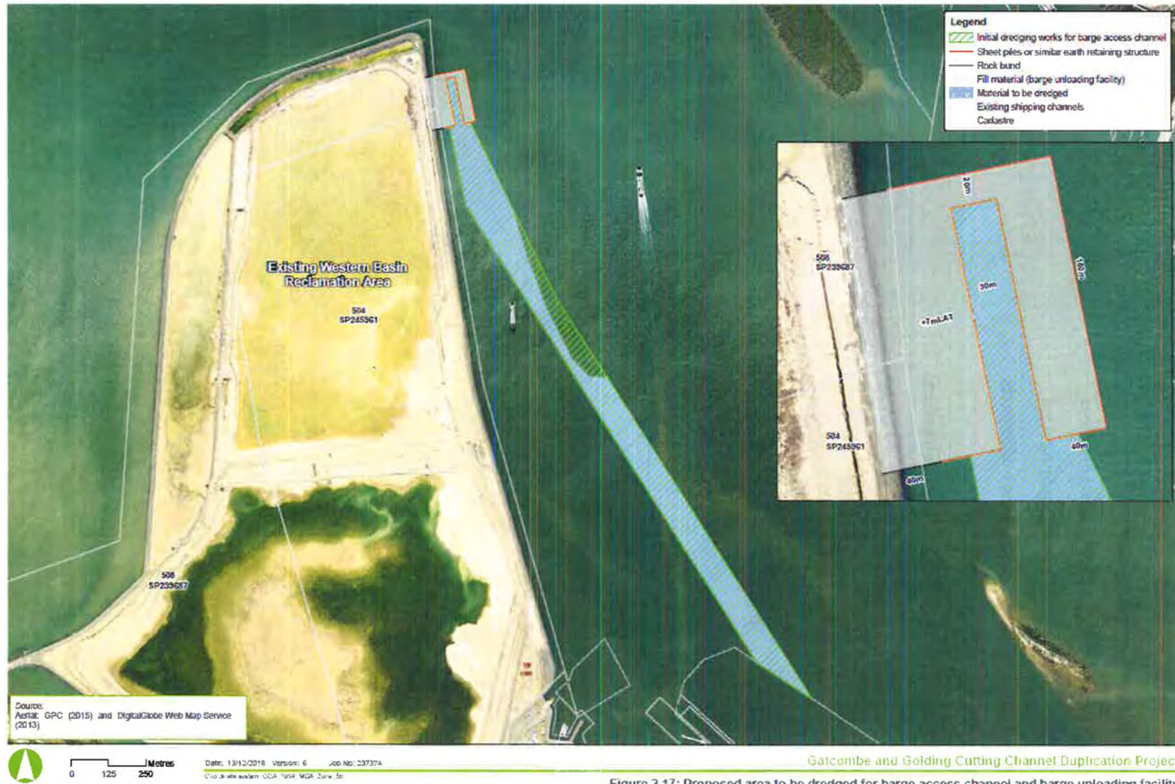
Figure 2.17: Proposed area to be dredged for barge access channel and barge unloading facility
