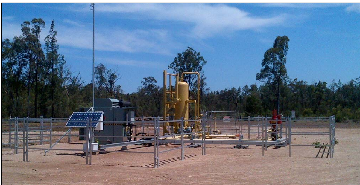
FIGURE 3-6: TYPICAL PUMPING WELL CONFIGURATION WITH WELLHEAD, DRIVE HEAD UNIT AND SEPARATOR
