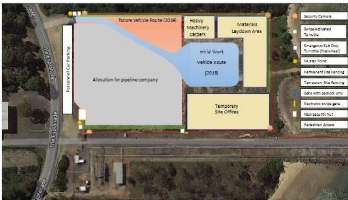
**Figure 1-2 : Indicative Site Establishment Layout (Rev C) Source: AGL, 2018**
