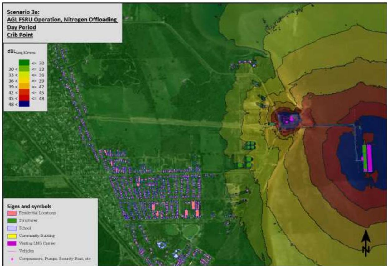
Figure C-2 : Noise modelling for regasification in progress (Day Period)
