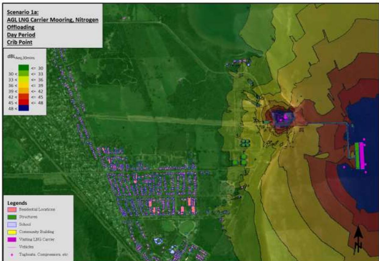
Figure C-1 : Noise modelling for mooring of LNG carrier (Day Period)
