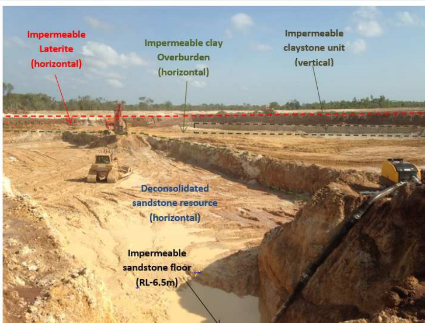
Photo of the 2013A extraction cell showing the site's geological sequence. The resource has impermeable laterite and clay overburden above; impermeable sandstone below; low permeability deconsolidated sandstone laterally; and larger scale impermeable claystone barriers laterally.
