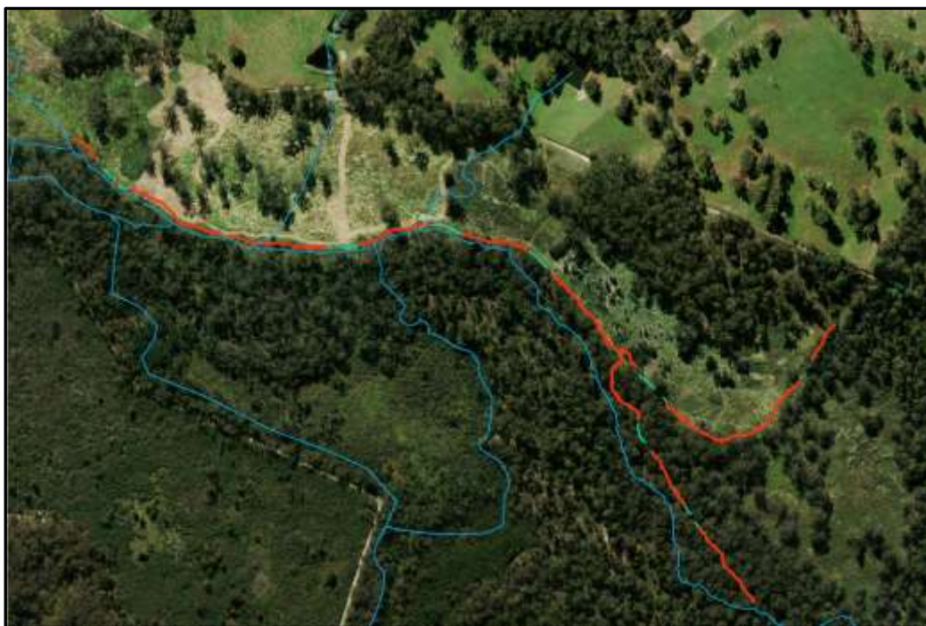
Figure 10. Areas of levee to be removed (shown in green) to permit floodplain inundation in the upstream desiccated parts of Cockatoo Swamp. Source: Claire Quinlan, Jacobs.
