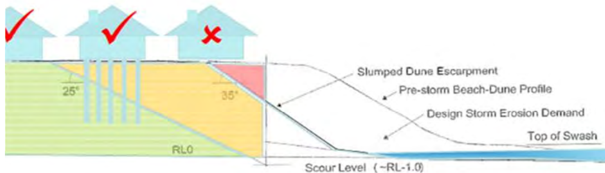
Figure 3-4 Using Foundation Piles to access the Stable Foundation Zone
