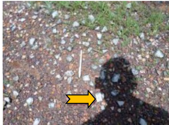
Photo 10. Section 32 – Area E1, external, north-west corner of 32 compound, debris – asbestos fibre cement sheet. Reference: 17069-001-028.
