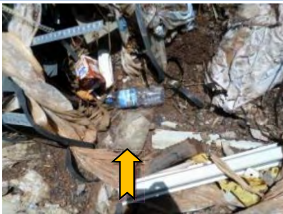
Photo 17. Section 32 – Wagait Landfill, external, north-west perimeter of landfill, debris – assumed asbestos fibre cement sheet.
