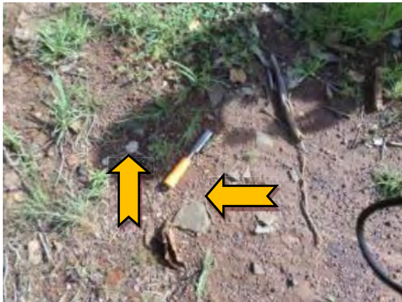
Photo 9. Section 32 – Area E1, external, east of 32 compound, debris – asbestos fibre cement sheet. Reference: 17069-001-028.
