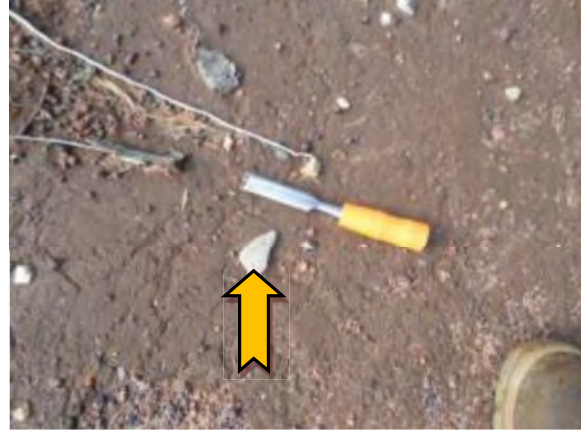
Photo 8. Section 32 – Area E1, external, west area, debris – asbestos fibre cement sheet. Reference: 17069-001-028.
