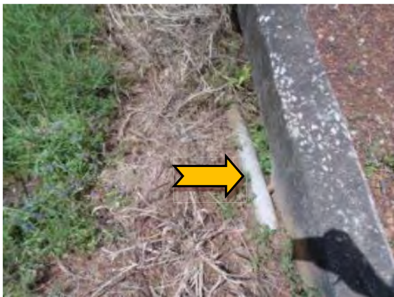
Photo 11. Section 32 – Area E1, external, east of 32 compound, pipe in drainage area – asbestos moulded fibre cement. Reference: 17069-001-028.
