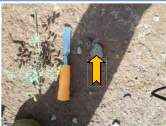
Photo 5. Section 32 – Area E1, external, south-east corner, debris – asbestos fibre cement sheet. Sample: 17069-001-027.
