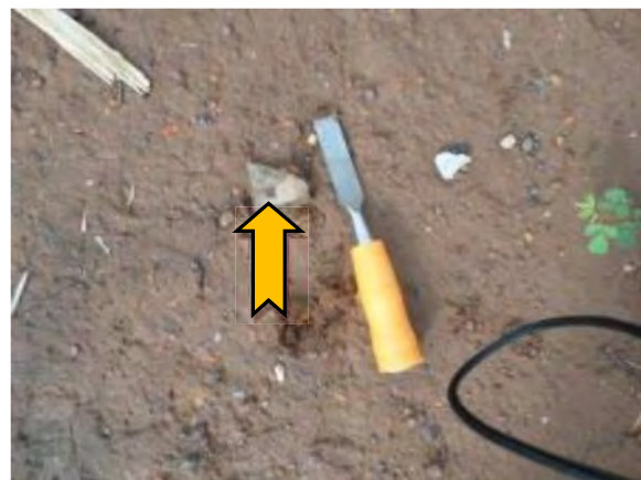
Photo 4. Section 32 – Area B, external, central area, debris – asbestos fibre cement sheet. Reference: 17069-001-026.
