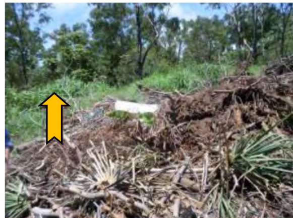
Photo 16. Section 32 – Wagait Landfill, external, south-east corner, debris – Assumed asbestos fibre cement sheet.
