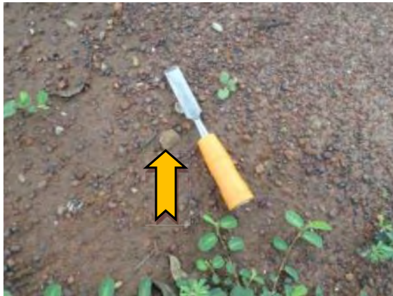
Photo 1. Section 32 – Area B, external, south-east corner, debris – asbestos fibre cement sheet. Sample: 17069-001-025.
