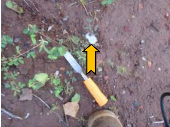
Photo 7. Section 32 – Area E1, external, north central area, debris – asbestos fibre cement sheet. Reference: 17069-001-028.
