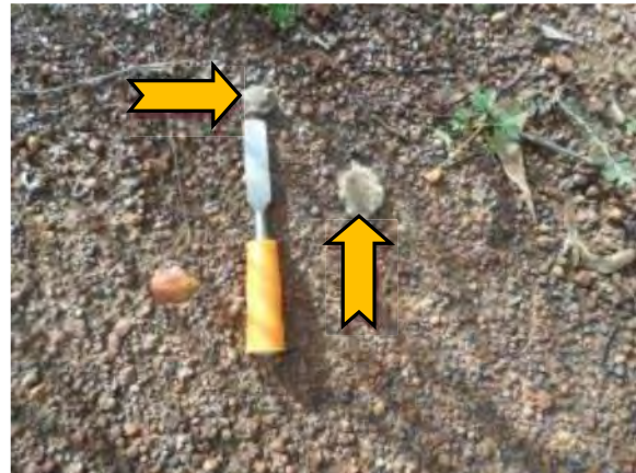
Photo 2. Section 32 – Area B, external, east area, debris – asbestos fibre cement sheet. Sample: 17069-001-026.
