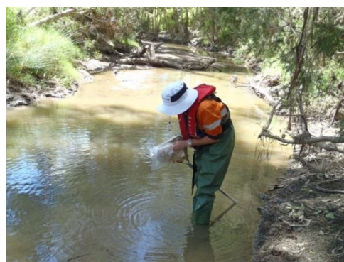
b) transferring the sample to the plastic bag for preservation
