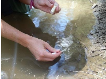
a) Collecting the sediment scrape
