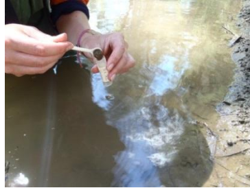
b) placing the sediment in the vial
