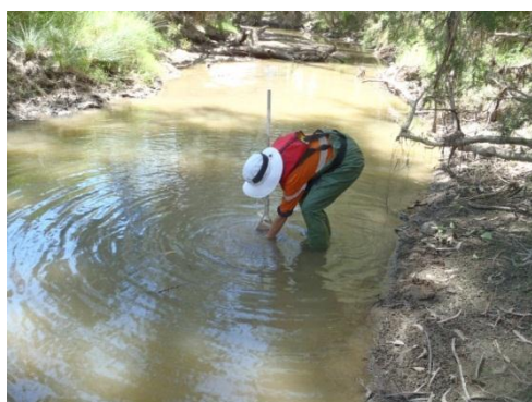
a) collecting a macroinvertebrate bed sample in soft sediment
