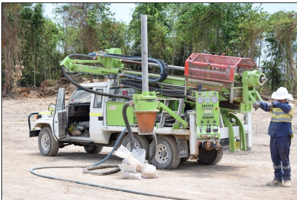
Figure 1. 4WD mounted Aircore Exploration Drill Rig
