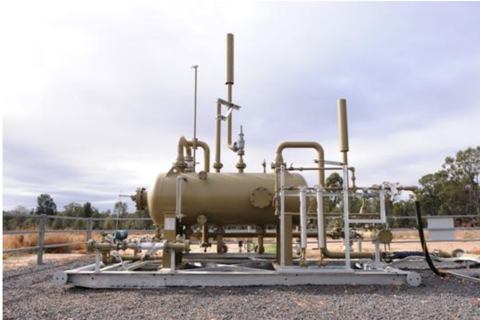
Plate 4: Typical Wellhead Separator
